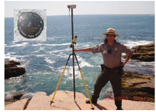
Figure 2. A park ranger uses a survey monument (beneath the center tripod leg), or benchmark, to position an RTK-GPS instrument. These monuments serve as stable reference points when collecting elevation data. Inset: Example of an embedded NPS survey monument, several inches in diameter. Photos courtesy of Michael Bradley, University of Rhode Island Environmental Data Center
