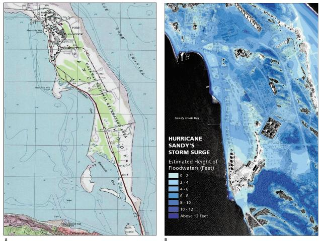
Figure 1. A. Contour map of southern Sandy Hook Bay on the New Jersey coast. The curved contour lines join points of equal elevation. Map courtesy of the United States Geological Survey. B. Inundation of the Fort Hancock area at Gateway National Recreation Area (GATE), NJ, as a result of Hurricane Sandy storm surge. The powerful storm resulted in several feet of flooding and damage across the Sandy Hook peninsula. Map courtesy of GATE GIS URI Branch
